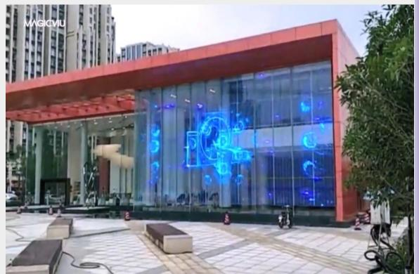
Transparent LED film is a high-end revolutionary selfadhesive thin film easily attached to any glass surface transforming a normal window or building façade into an eye-catching display quickly and with minimum efforts.
