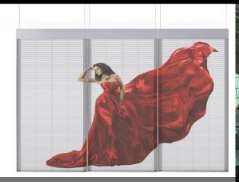
Transparent LED Screen is a type of LED display screen that is clear like a glass (60%-85% transparency) and has functions of an LED. It enables the viewers to see whatever is shown on the glass along with providing a complete coverage of its background as well. Since it enables audience to see what is happening behind the screen, it is also referred to as a see-through screen.
