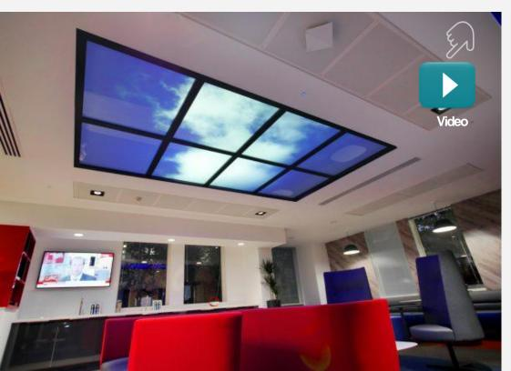
Using ultra short projection technology we are able to fit the screen into a very low ceiling void with only 450mm between the screen and the slab above.
